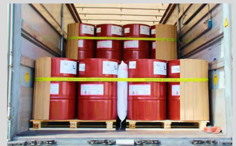
5. complete loading. Fill gaps with dunnage bags
