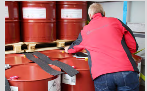
3. double deck loaded. Place anti-slip mats underneath
