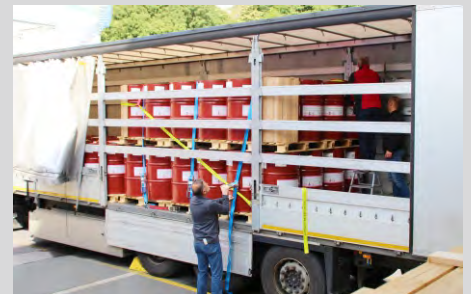
4. lash down the double deck. Use edge protection
