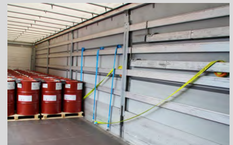
2. hook in Truck Lash, fix it to the drop sides
