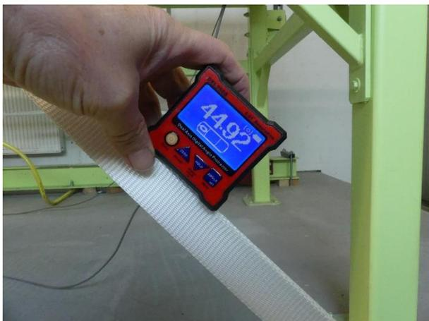
Abb. 3 Verlauf/Winkel ( $\alpha = 43-46^\circ$ ;  $\beta = 80^\circ$ )
