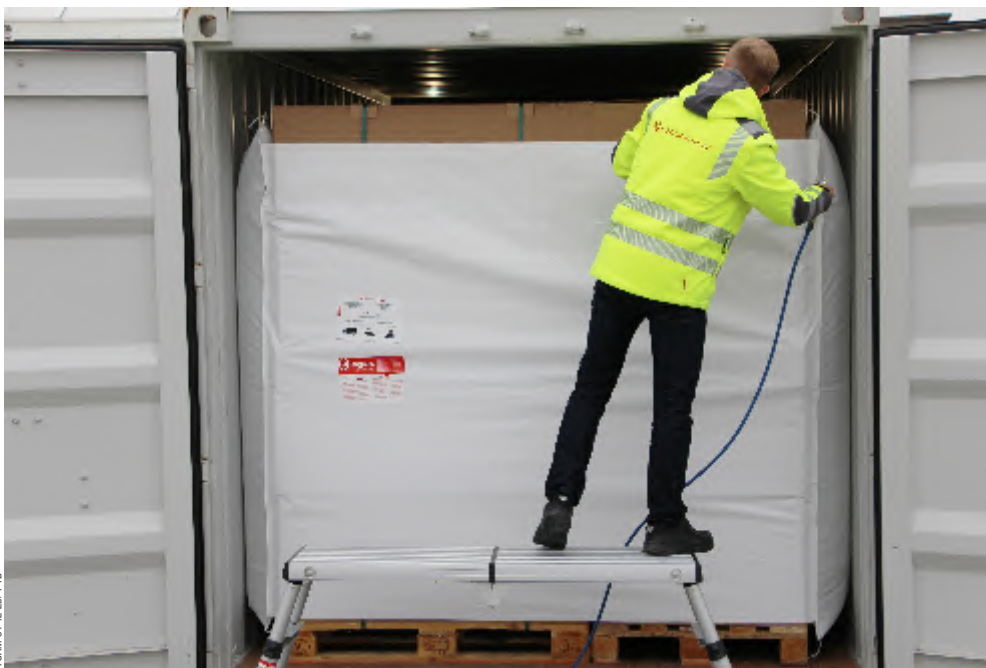
Tilt test up to 53° inclination
