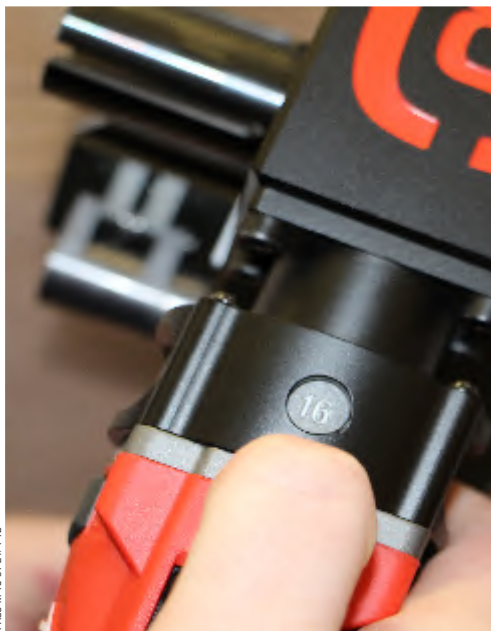
adjustable torque for reproducible pre-tensioning forces
