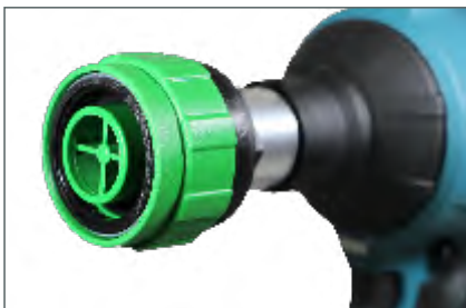
Quick Connect directly screwed onto the device
