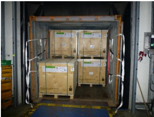
Fig. 3: Stowing the wooden crates up to the door
