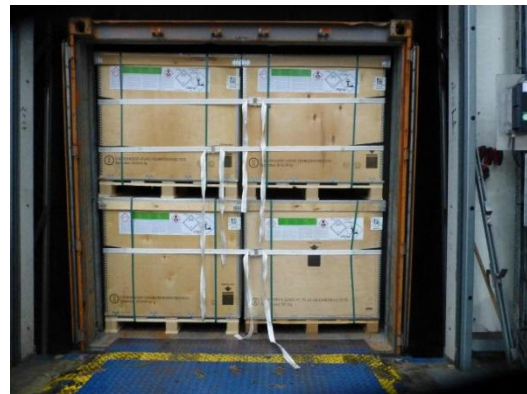
Fig. 4: Closing the restraint system
