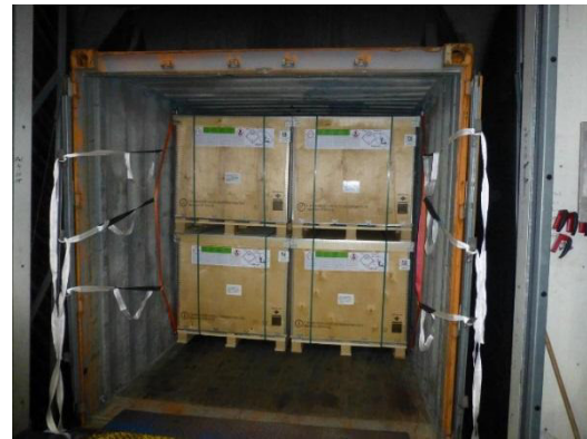
Fig. 2 Preparation of 3-piece lashing
