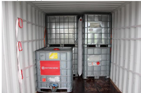
Fig. 4: Form-fit stowage in container offset by 90°
