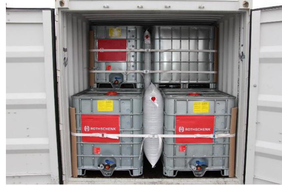
Fig. 6: Finalizing lower lashings with 1/4 shells
