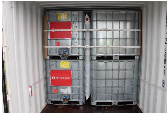
Fig. 5: Finalizing upper lashings with 1/4 shells
