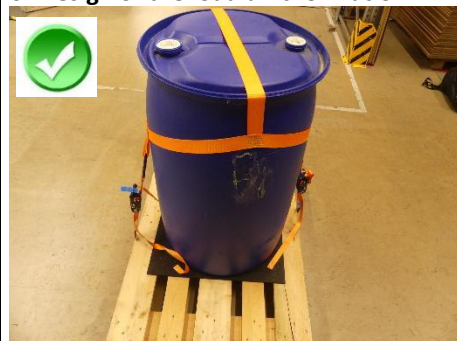
Fig. 1 and 2: Metal drum with PET strap and PE drum with polyester strap and metal hook fixation
