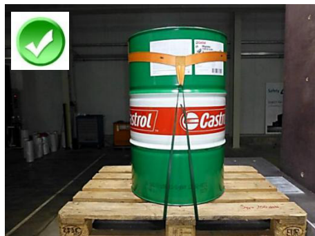
Fig. 1 and 2: Metal drum with PET strap and PE drum with polyester strap and metal hook fixation
